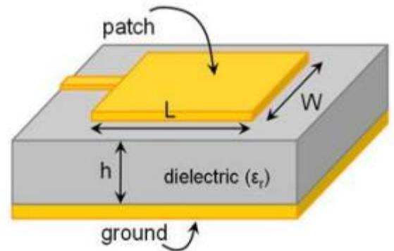
Figure 1: Structure of a Microstrip Patch Antenna
