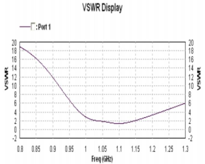
**Figure 4:** VSWR Display of rectangular microstrip patch antenna.
