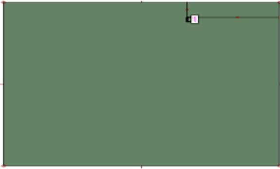
**Figure 2:** Rectangular microstrip patch antenna resonating at 1.09 GHz.
