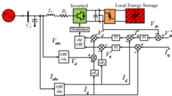
Fig. 5. The control strategy of utility interactive inverter during grid-connected mode.
