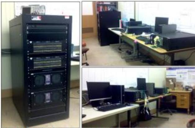
Fig. 3. Real Time HIL System for Simulation of Power Systems.
