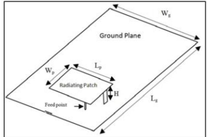
Fig. 1: Basic PIFA Structure
