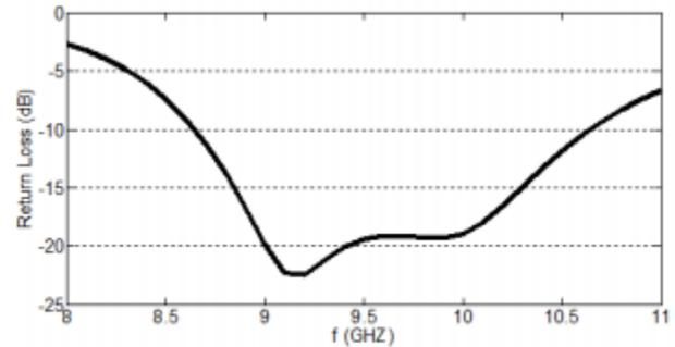
Fig. 2 Return Loss of single element
