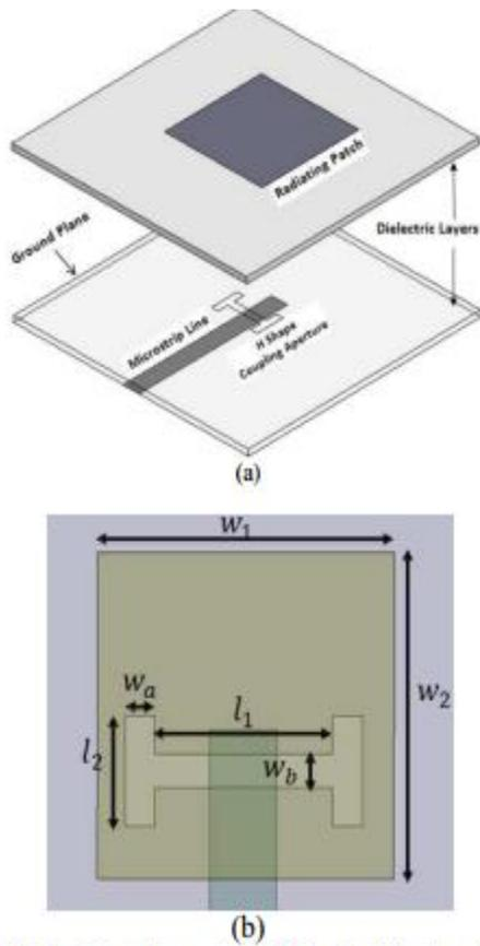
Fig. 1 Configuration of ACMA a) side view b) top view  $l_1 = 4.8\text{mm}, l_2 = 2.7\text{mm}, w_1 = w_2 = 8\text{mm}, w_a = w_b = 0.8\text{mm}$
