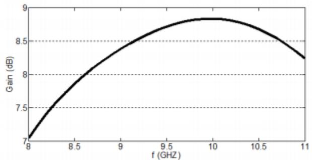
Fig. 3 Gain of single element
