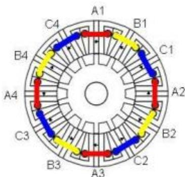
Fig. 1. Cross section of a 12/14 pole machine.
