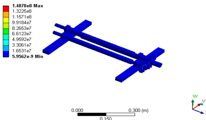
The equivalent (von misses) stresses results shows that there will be max stresses at red portion and minimum at blue portion
