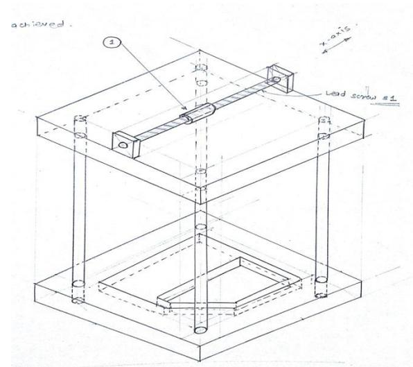
Fig. 4.4: Isometric view of machine assembly (satisfying x-axis motion requirement)
