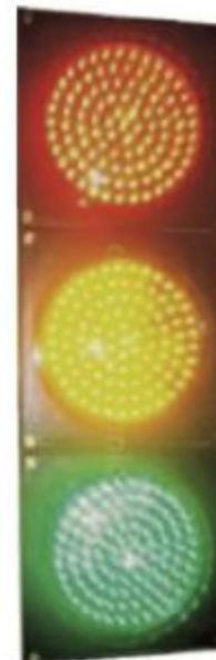
Fig. 4 – Illumination of LED based traffic lighting system.
