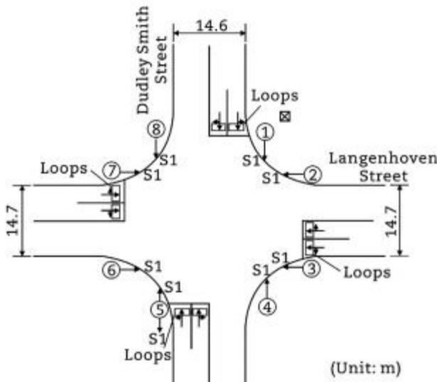
Fig. 2 – A typical 4-way junction.
