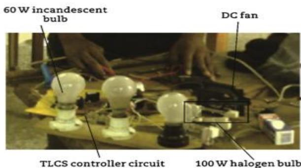
Fig. 6 – T-junction experimental setup at power-off mode.
