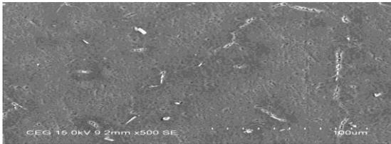
Fig-8:SEM micrograph of Mica 3% composition
