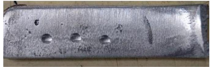
Fig-4: Hardness test specimen
