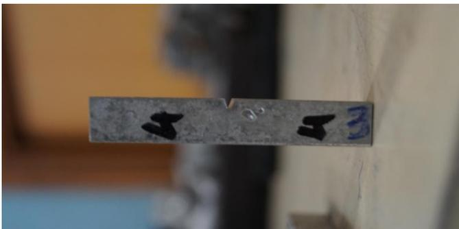
Fig-3: Impact test specimen
