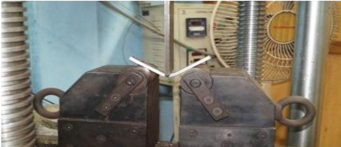
Fig-2: Flexural test specimen
