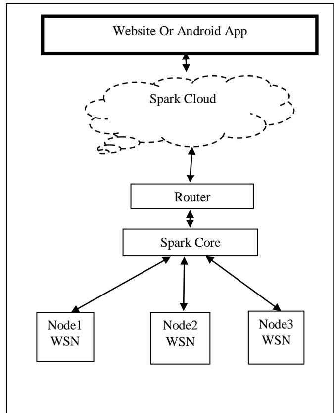
Fig. 1. Block Diagram of Internet of Things using Spark Core
