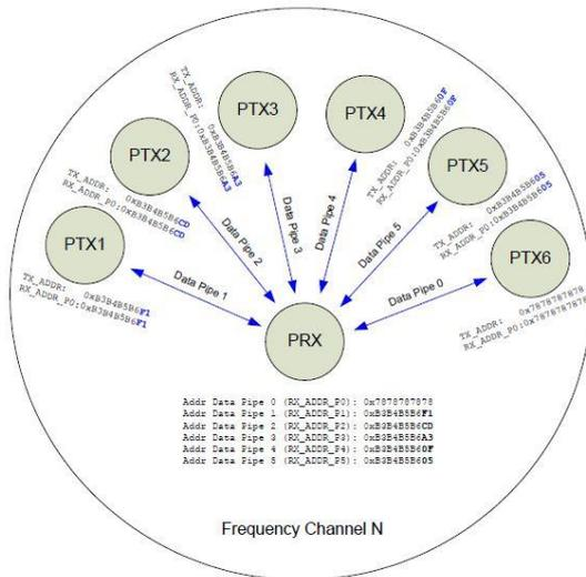
Fig. 2. Pipelined Architecture
