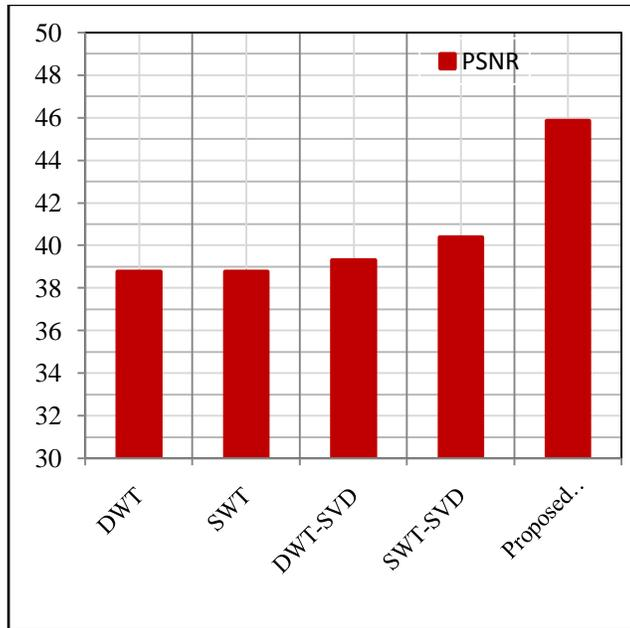
Figure4. Comparison of PSNR for various watermarking approach
