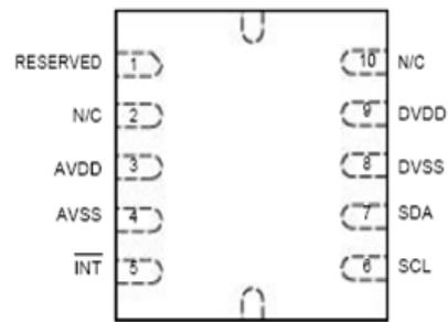
Fig.4 MEMS PIN Configuration
