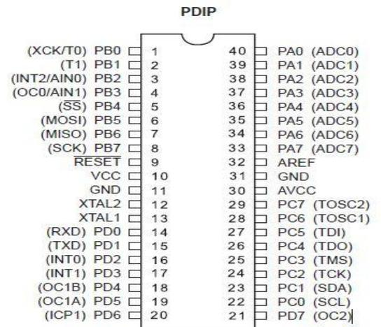
Fig 3: Pin Configuration ATmega 16
