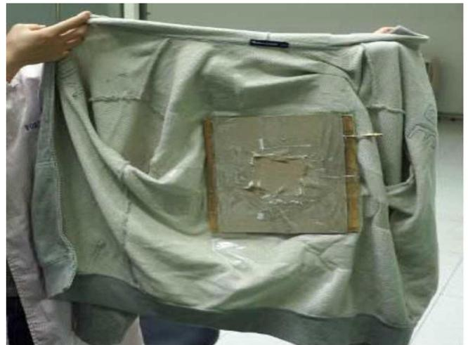
Fig.- 6: Antenna Implanted on Cloth
