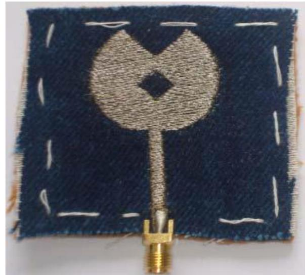
Fig. 9: Embroidered Wearable Antenna Prototype
