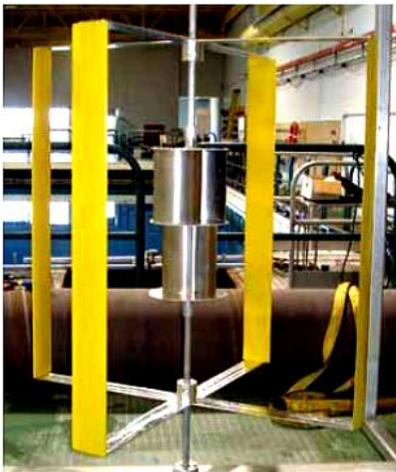
**Fig- 12: Hybrid configuration of Darrieus and Savonius rotor**
