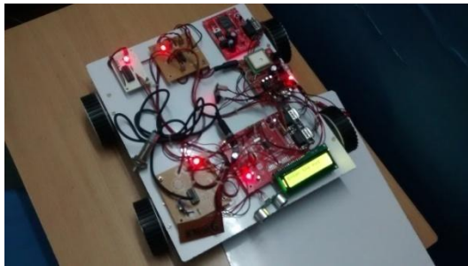
Fig .6.Robot section developed for detecting explosives
