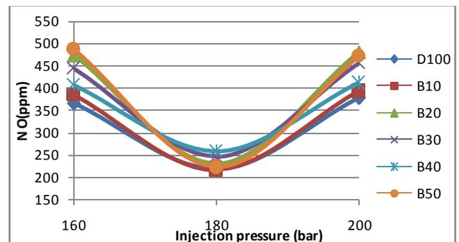
**Fig-7: Variation in Oxides of Nitrogen (NO) with Injection pressure**
