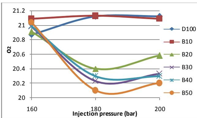
**Fig-9: Variation in Oxygen (O2) with Injection pressure**
