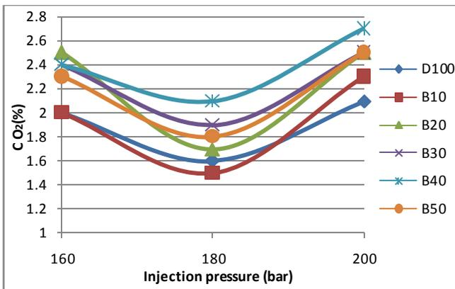
**Fig-8: Variation in Carbon dioxide (CO2) with Injection pressure**
