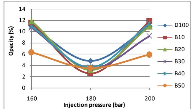
**Fig-10: Variation in Opacity with Injection pressure**
