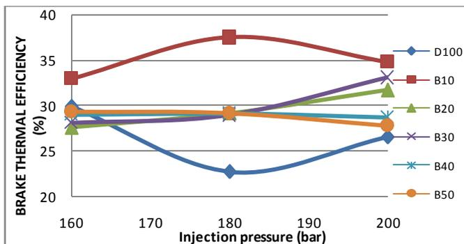
Fig-5: Variation of Brake Thermal Efficiency with Injection pressure
