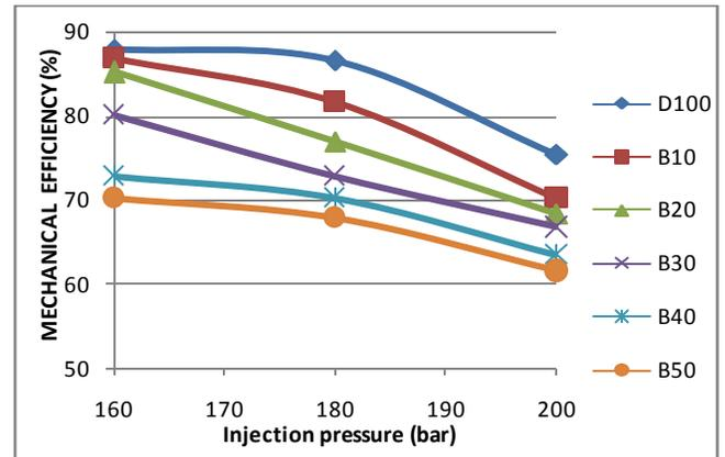
Fig-6: Variation of Mechanical Efficiency with Injection pressure
