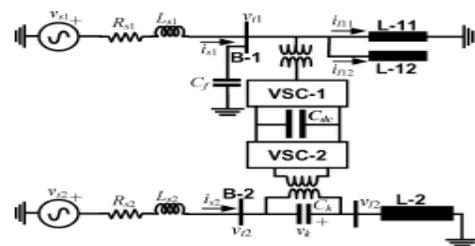
**Fig. 3** Typical IUPQC connected in a distribution system.
