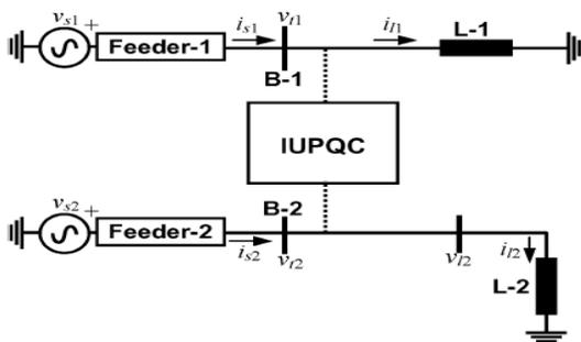
**Fig.1** Single-line diagram of an IUPQC-connected distribution system.
