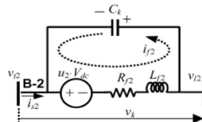
Fig.11 The equivalent circuit of the VSC-2
