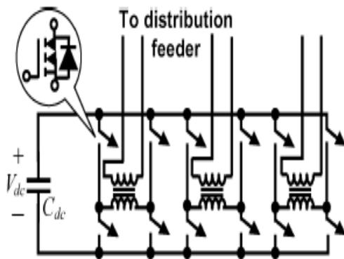
Fig.4 Schematic structure of a VSC.
