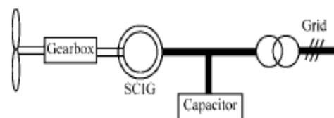
Figure: 3. Fixed speed concept using a multistage gearbox
