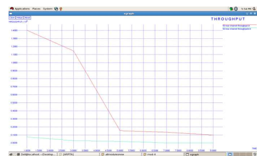
Figure 4. Throughput Graph for 50 nodes of MMAC using AODV and DSDV Routing Protocol
