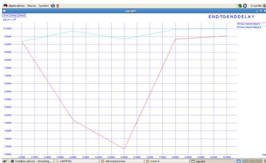
Figure 7. End to End delay Graph for 50 nodes of MMAC using AODV and DSDV Routing Protocol
