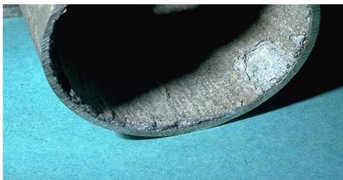
Fig-5: Intergranular corrosion of metal
