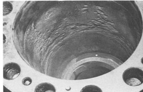
Fig-7: Erosion corrosion of metal
