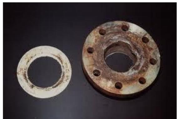
**Fig-3:** Crevice corrosion of metal
